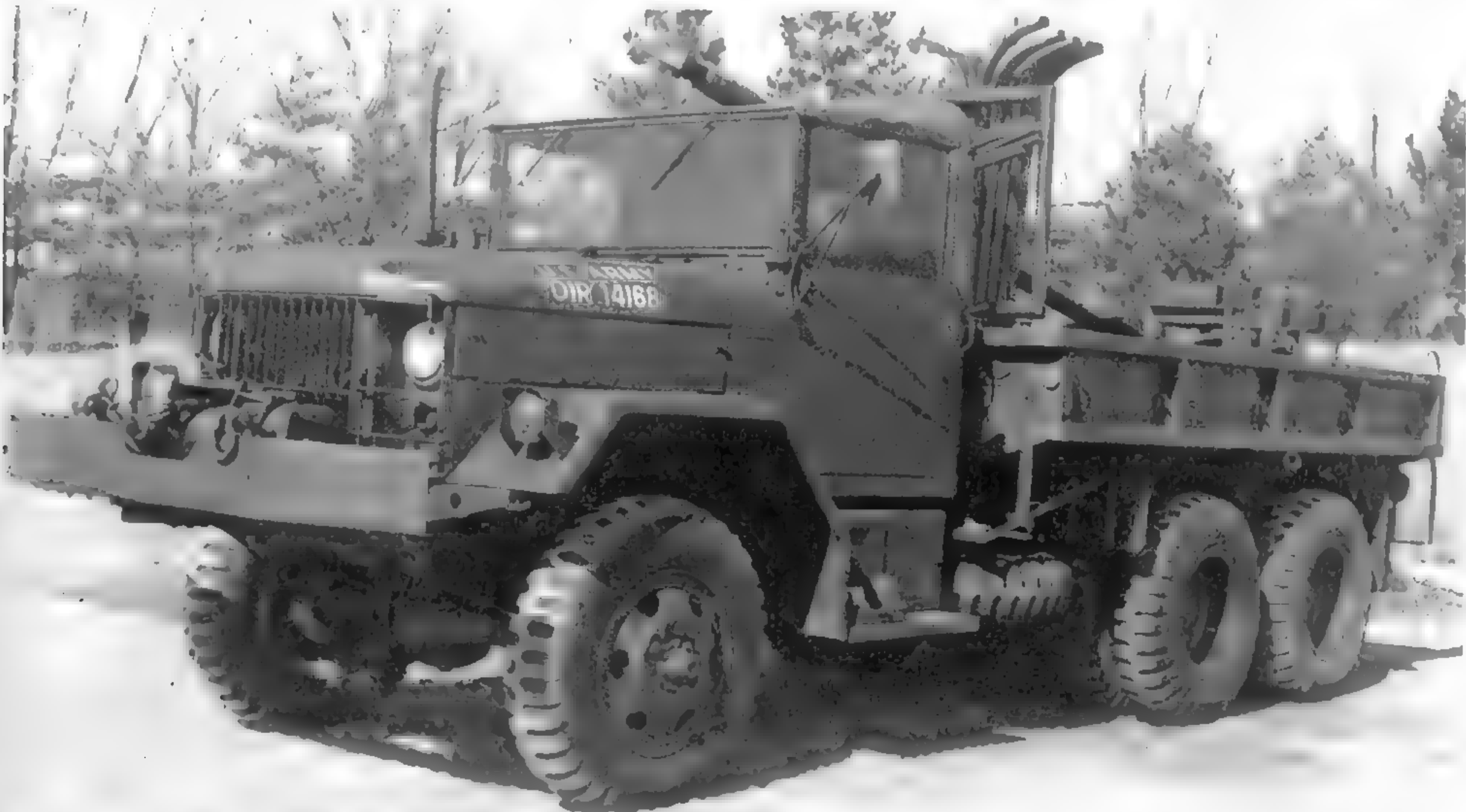
The M764 was the improved model pole setter/earth borer. In addition to a multi-fuel-powered dual wheel chassis, it had a more modern boring machine and hydraulic outriggers. (U.S. Army photo)
